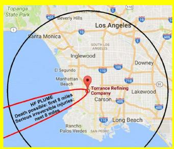
Representation of the ground-hugging acid cloud from 50,000 lb of modified hydrofluoric acid (MHF) very nearly released during the 2015 Torrance refinery explosion. The prevailing wind that day was toward the west.
